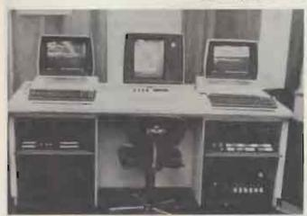
Astrotek 2000. The processors and disk drives are housed in cabinets under the table. Here the two doors have been opened to reveal the operator controls. These are Model 40 terminals, but PCs could be used. In the center is the noninteractive GDT preview monitor, which displays paginated text.
