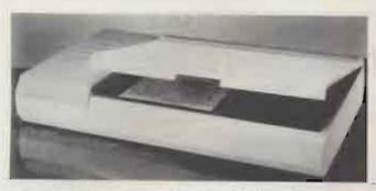
Ana Tech 1760 Corporate Scanner. The first tabletop, highresolution scanner to offer built-in raster-to-vector conversion.
